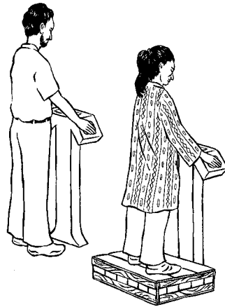
A platform can also make it easier for shorter people to reach switches, controls, and handles comfortably.
